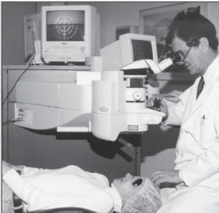
The VISX System Excimer Laser: developed by Dr. Stephen Trokel, to correct patients' vision without glasses, lenses, or invasive surgery.
